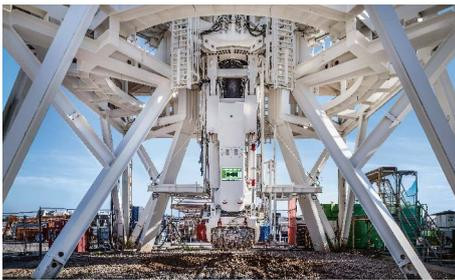
The Shaft Boring Roadheader's (SBR) telescopic boom and cutting drum.
