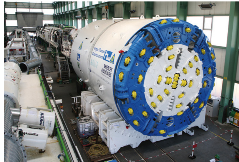
▼ Due to the changing ground conditions along the tunnel route, the contractor opted for a Multi-mode machine from Herrenknecht.
