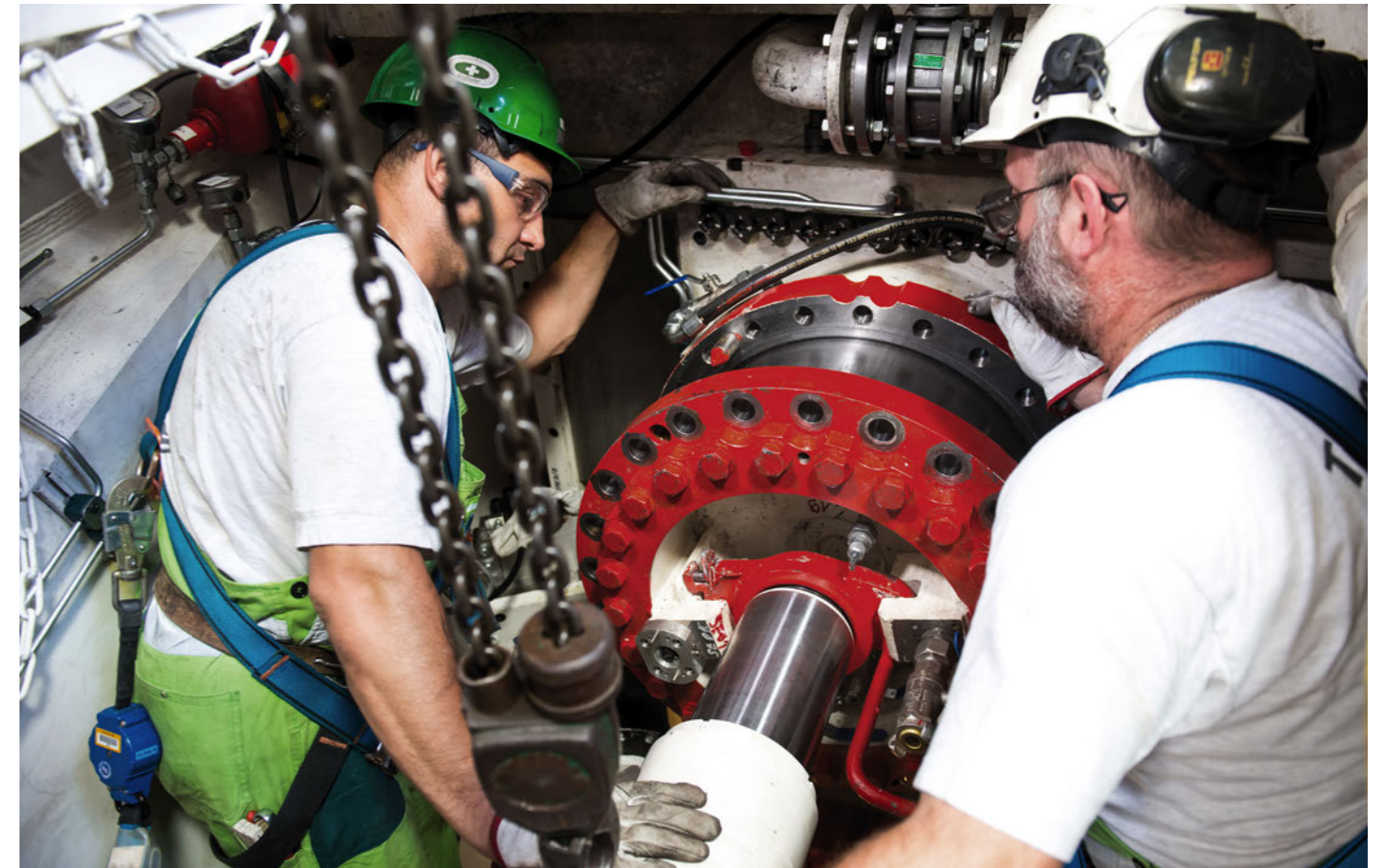
▲ During assembly in Germany the further developed lock systems for the disc cutters were extensively tested.
