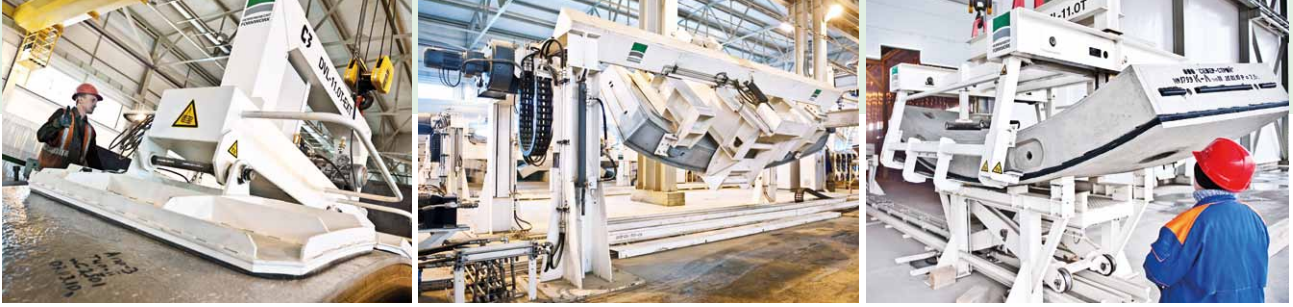
Handling equipment from Herrenknecht Formwork moves segments weighing several tonnes.
